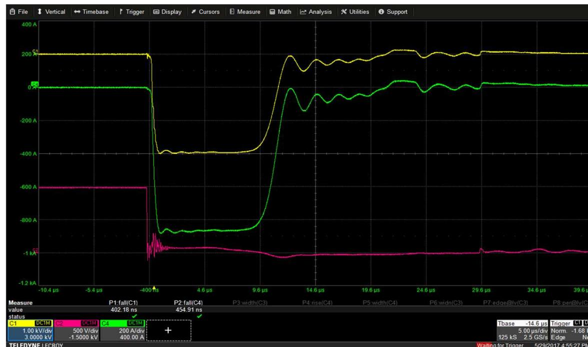
CH1 (Y) : PFN Output Voltage -3kV 1kV/div. 6kV charging 200pps
